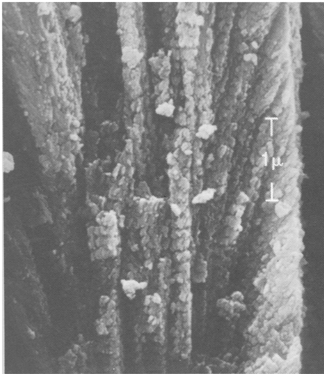
Fig. 11 Photomicrographs showing grain substructures resulting from rotation effects. (a) 0.18 \mu\text{m}/\text{rev} . (b) 2.6 \mu\text{m}/\text{rev}
